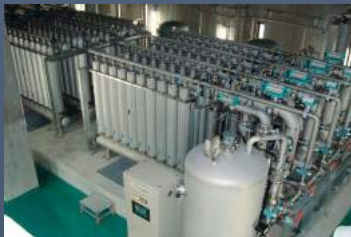
Water and Gas Membrane Separation (START)
